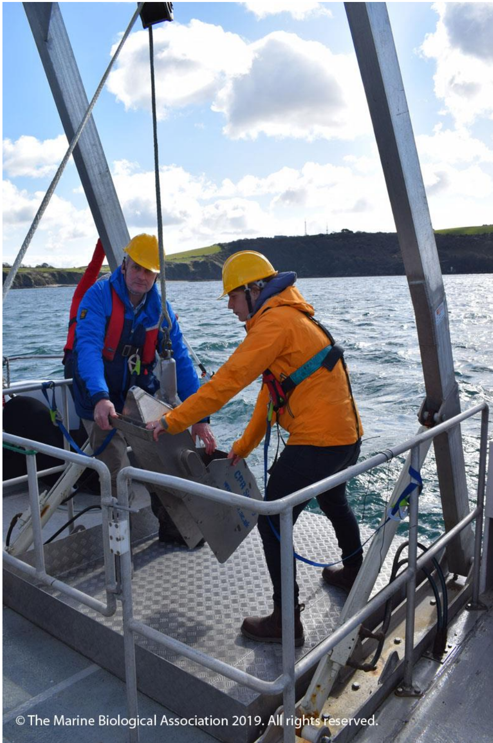
Professor Richard Thompson and Dr Ostle deploy the continuous plankton recorder (CPR).
